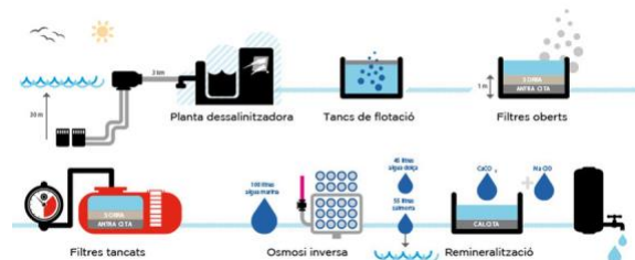
Figure 8. Desalination treatment process at the El Prat de Llobregat ITAM. Note. The schematic shows seawater capture, pretreatment, reverse osmosis, remineralisation and distribution to the Font Santa reservoirs. [17]
