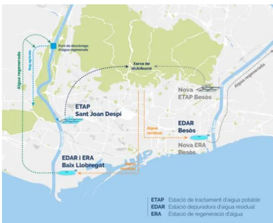
Figure 10. Current and planned wastewater, reclaimed-water and drinking-water distribution in metropolitan Barcelona. Note. The map shows the connection between the Baix Llobregat reclamation plant, the Llobregat River and the Sant Joan Despí drinking-water treatment plant. [15]
