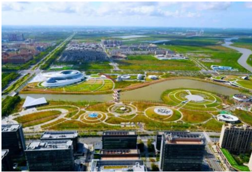
Figure 14. Lingang New City as a sponge-city pilot zone in Shanghai. Note. The image illustrates blue-green infrastructure used to absorb, store and reuse stormwater. [41]
