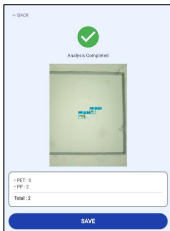
Figure 23: Microplastic detection and classification results displayed by the processing system
