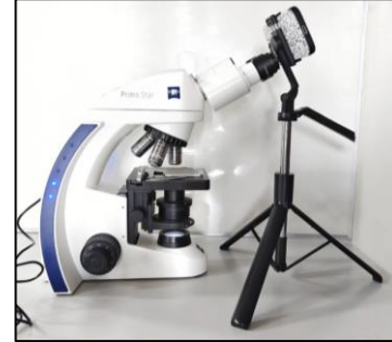
Figure 6: Experimental setup for Deep Learning model training data collection
