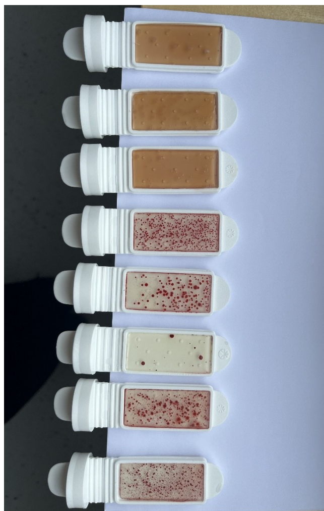
Image 1: Growth of bacteria on DipSlide TVC and Redspot / Coliform agar after incubation
