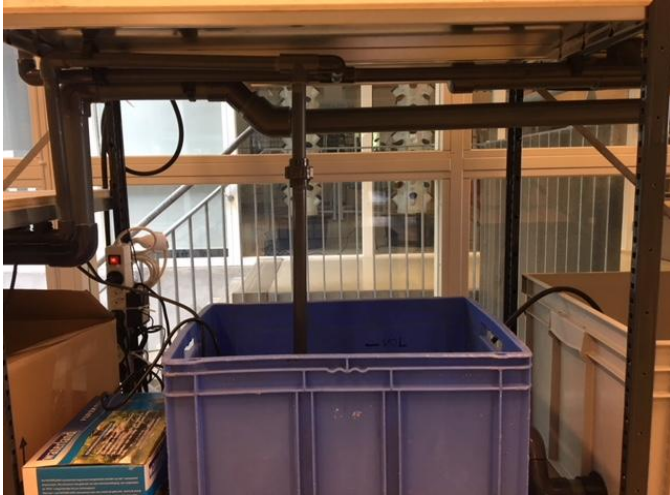
Figure 10: In this tank the water level is monitored and here lies the heating element, because we maintain tropical fish in our aquaponic system
