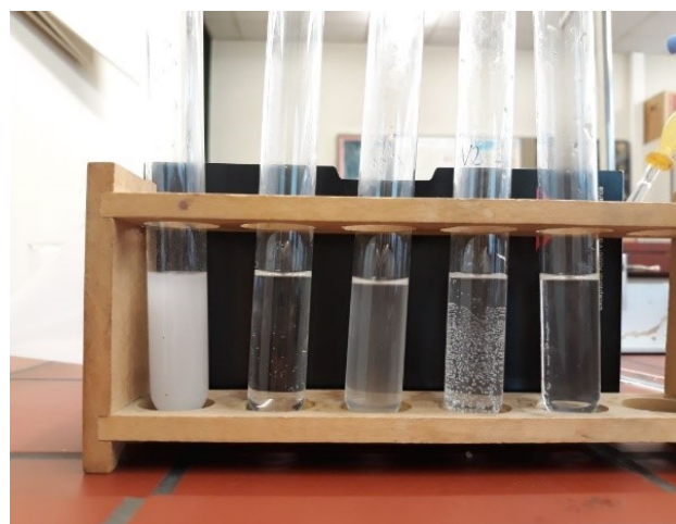
Figure 13 Sulfate test: From left to right: Ensinger, Black Forest, Gerolsteiner, Adelholzener, tap water
