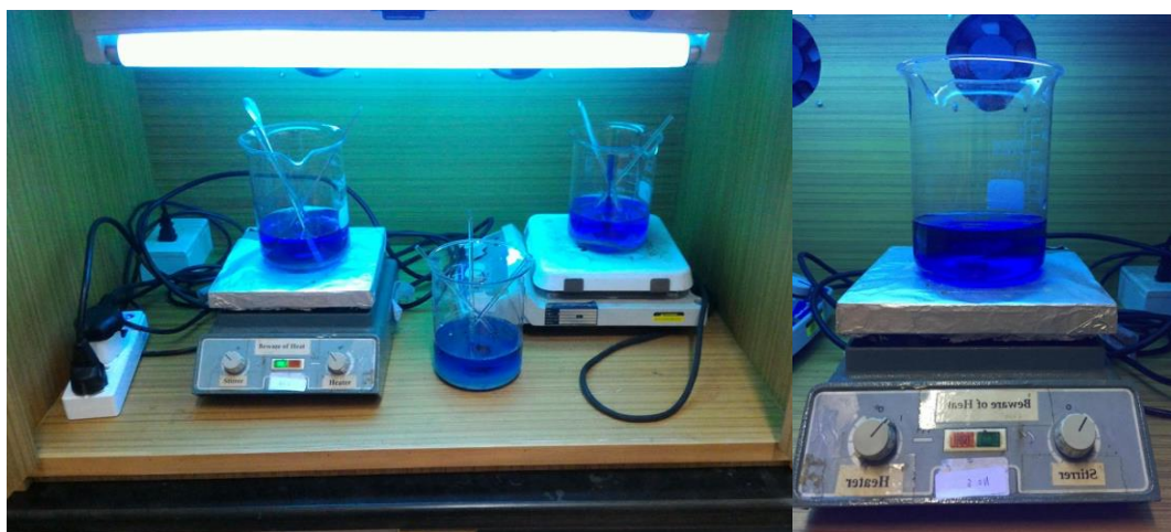
Fig: 2.2 Glass bowl reactor with magnetic stirrer on lab scale
