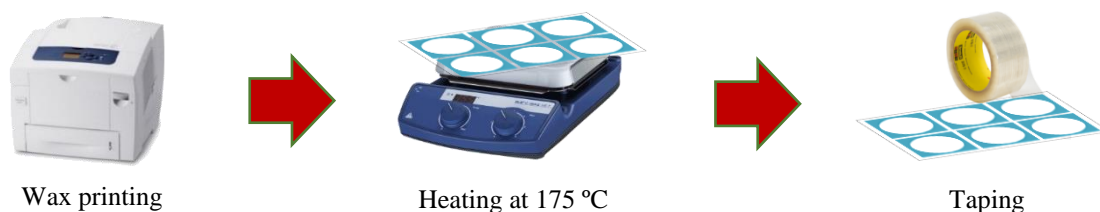
Fig. 5 Preparation of paper by wax-printing, heating, and taping
