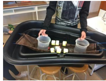
Figure 35: Testing the weight that the mesh could support.
