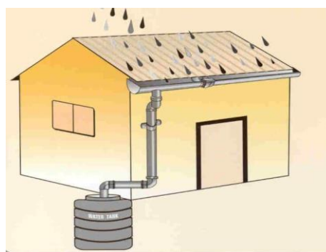
Figure 6: Very basic rainwater harvesting setup
