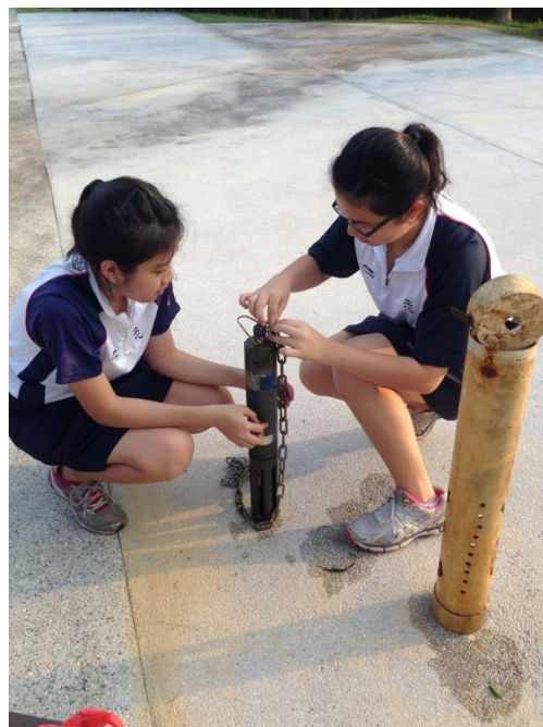
Figure 14: Priscilla (left) and Jing Yuan (right) preparing the YSI Datasonde for the downloading of data. Cylinder beside Jing Yuan is a protective casing for the YSI Datasonde when it is submerged in the pond.
