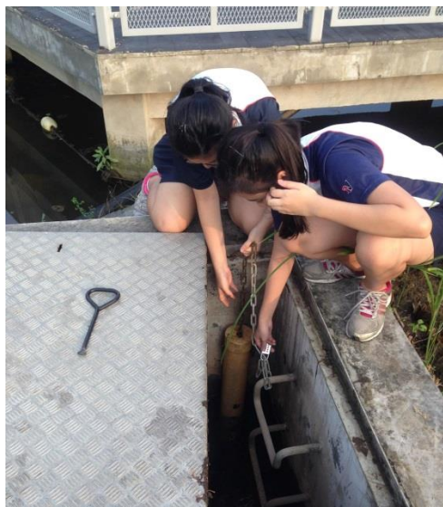
Figure 13: JingYuan (left) and Priscilla (right) unlocking a YSI Datasonde from the Site 3 manhole.
