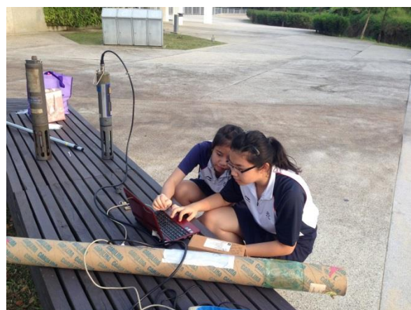
Figure 15: Priscilla (left) and Jing Yuan (right) using a laptop to download data from a connected YSI Datasonde.
