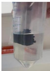
Figure 15: Separation of MCB using a magnet
