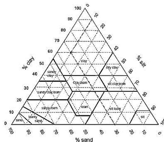
Figure 3. Example of soil triangle, which is used to determine the type of soil of a certain sample by using the percentage shares of every layer and drawing lines.
