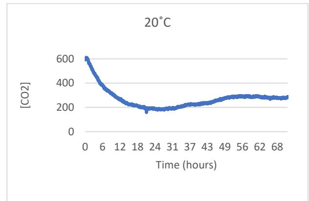
Figure 9: Test at 20°C with algae
