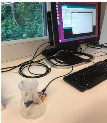
Figure 6: the meter in the erlenmeyer connected to the computer
