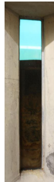
Figure 8: Filter with different layers (profile view)
