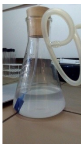
Figure 11: Sulphite and calcium sulphate decanting on the bottom of the Kitassato.
