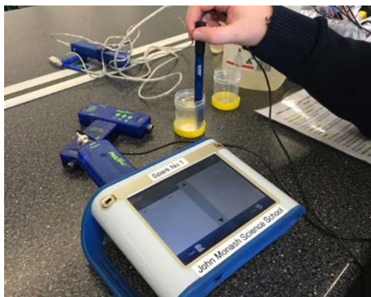
Figure 2: Analysing water samples using PASCO SPARKView Source: Musgrave 2018
