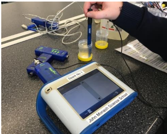
Figure 7: Analysing water samples using PASCO SPARKView Source: Xu 2016
